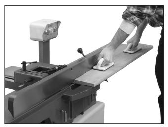
Figure 34. Typical rabbet cutting operation.
